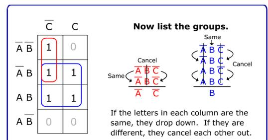
Fig. 3. Snapshots on Simplification by K-MAP in Digital Circuits course mentioned by students as one of the concept made easier by animations.
